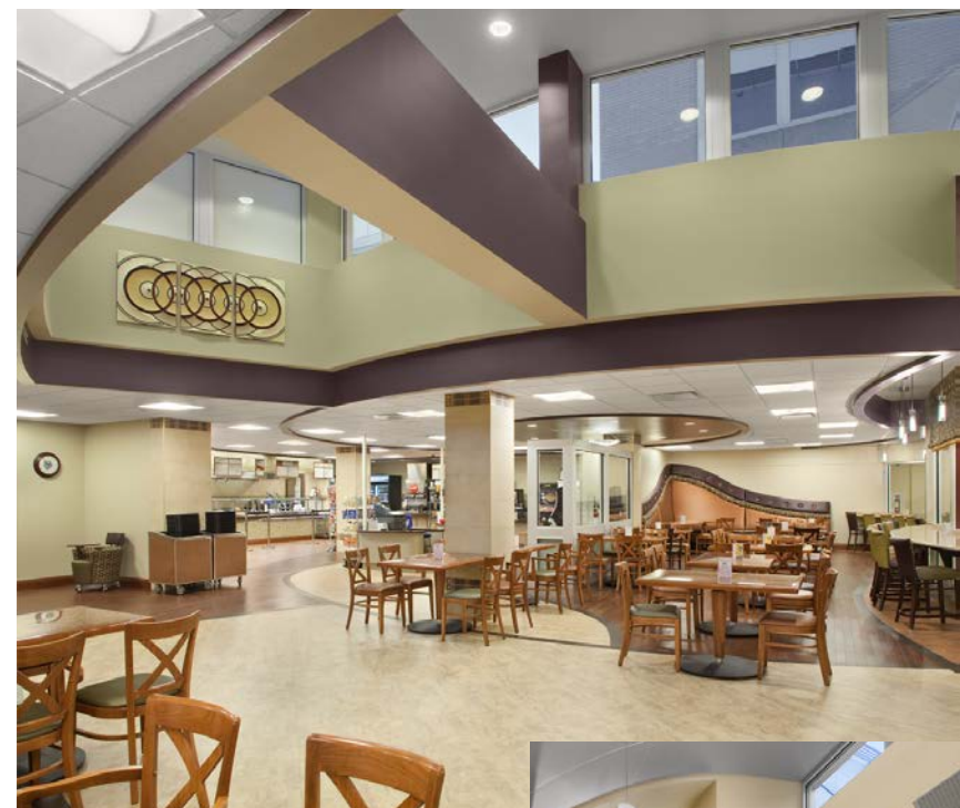
VA Wade Park Facility Canteen Kitchen Renovations added new food court concessions along with a spacious dining area located under an impressive new clerestory. The addition of the clerestory was a challenging task as it required proper shoring of the existing roof deck, and structural changes underneath in order to keep the operating departments below completely watertight throughout the project.
